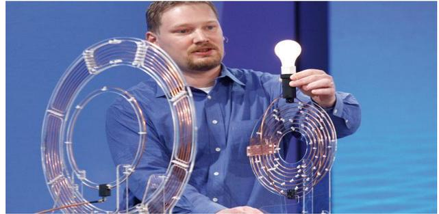
Fig. 8. Experiment at MIT for WPT.
